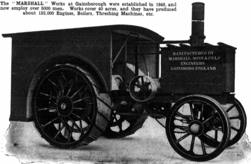
The above shows a 32 H.P. Draw Bar and 60-70 Brake H.P. Tractor. One Speed.
