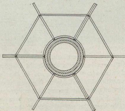
Vertical section of chimney, jacket, and cylindrical iron form with staging.
