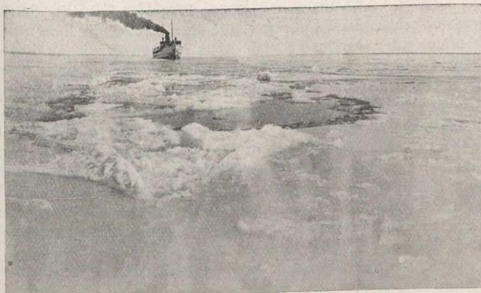
**Fig. 9.**—C.C.S. "Lady Grey" backed down the channel ready to come forward full speed into the ice. The V groove of the ship's prow may be seen in the foreground. The smoke of the "Montcalm" may be seen on the horizon.
