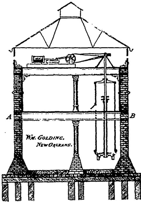
the water from the pit, and deliver it into the tank, from which it flows to the out-fall receptacle. The bottom of the tank is placed on a level with the minimum height of the out-fall receptacle, while the top of the tank will be placed above maximum height of out-fall receptacle.
