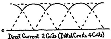
Direct Current 2 Coils (Dotted Curves 4 Coils)
