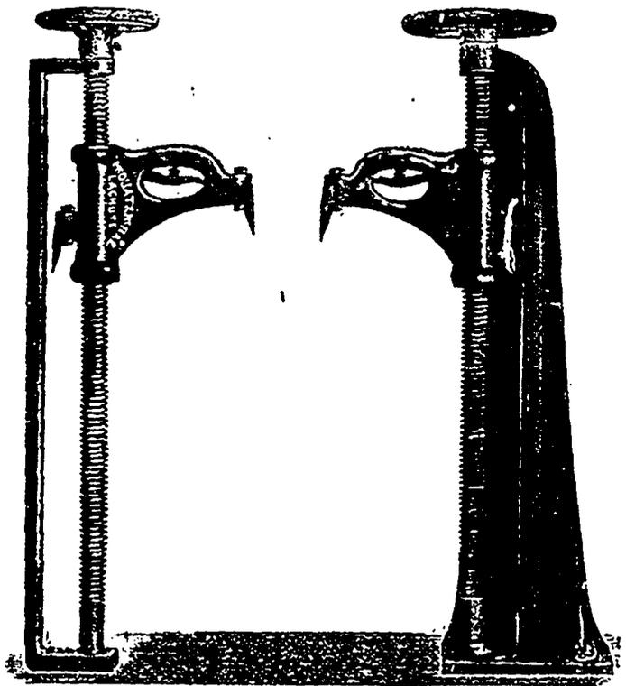
will send it into position in the log. Then by simply pressing a latch, it is instantly released without the use of a hammer. The advantages of these points are manifest to every sawmill man, and no other frost dog will accomplish these results.
