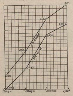
the test pieces being composed of 1 part of cement, 3 parts of normal sand, 2 per cent. of plaster of Paris, and 8 per cent. of water.
