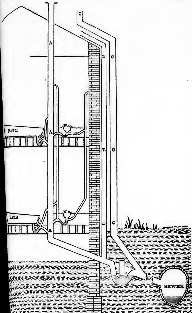
A-Extension upwards of soil pipe.
