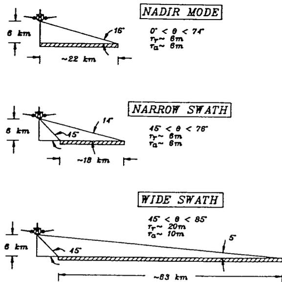
Figure 1: Radar Imaging Modes.
