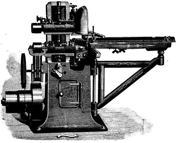
This is an entirely new style of Tenon Machine. The frame is cast in one piece, and the working parts stand solidly on a pedestal avoiding
