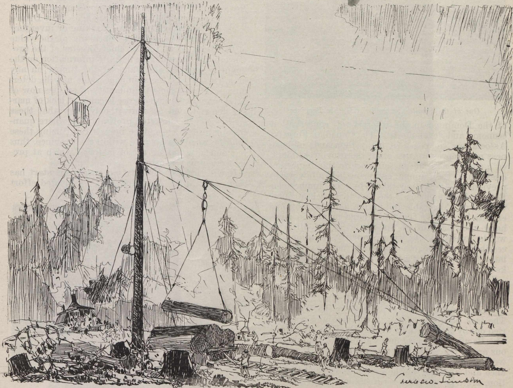
Moving Big Logs by means of the "High Lead" in B.C.; from a drawing by Chas. W. Simpson, R.C.A., by kind permission of the Christian Science Monitor.
