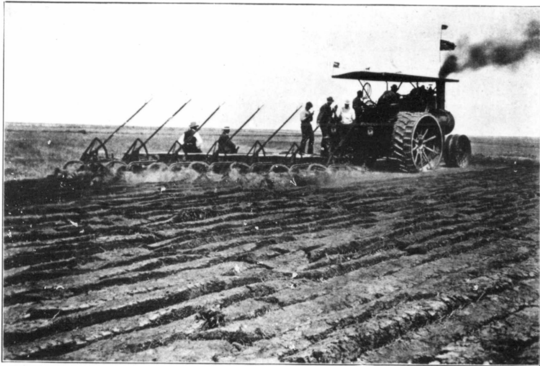
As it was pulled at the Winnipeg Motor Contest by a Rumely 35 Horse Power Steam Engine. (Bronze medal winner class C steam engines.)
