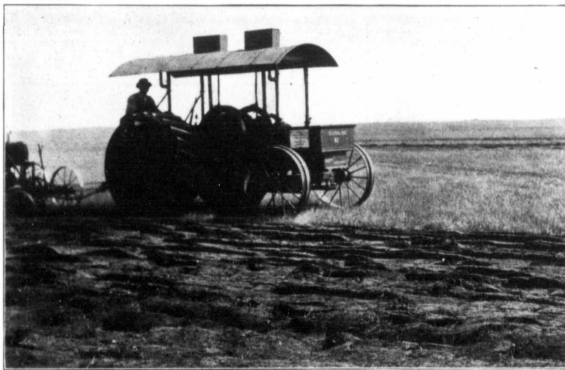
Goid Shapley & Muir 20 h.p. Gas Tractor in the contest. This engine pulled 3, 2 bottom 14 in. Imperial Gangs. The photographer miscalculated and mapped only the engine at work
