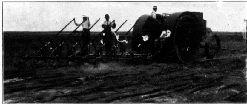
25 h.p. Gas Traction Engine pulling a 6-Bottom 14-Inch Cockshutt Engine Gang.
