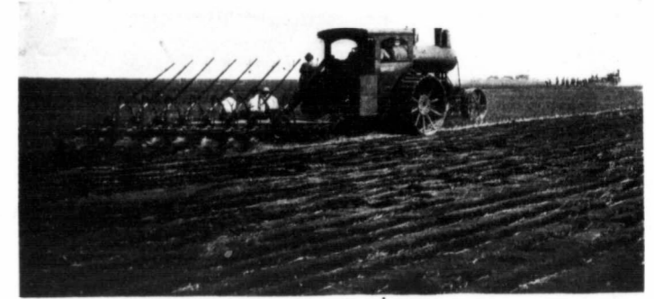
Plowing with the Avery 20 h.p. Double Undermounted Engine, and Pulling 8 14-inch Plows. One of the very best jobs of Plowing in the Contest
