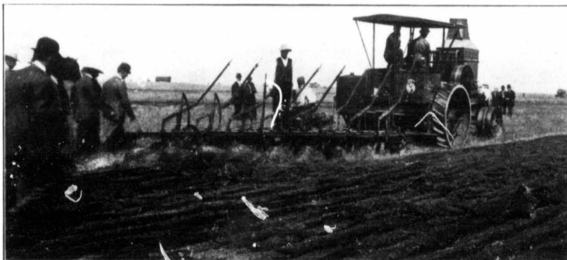
The Rumely Oil Pull Kerosene Tractor Pulling a Rumely 8 Bottom 14-Inch Engine Gang
