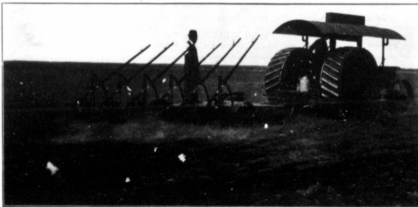
The Gookl, Shapely & Muir 30 H.P. Gas Tractor Pulling an 8 Bottom 14-Inch Cockshutt Engine Gang
