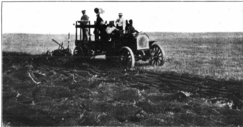
The Avery Tractor Pulling a 3 Bottom 14-Inch P. and O. Gang. The Little Tractor Attracted No Small Amount of Attention
