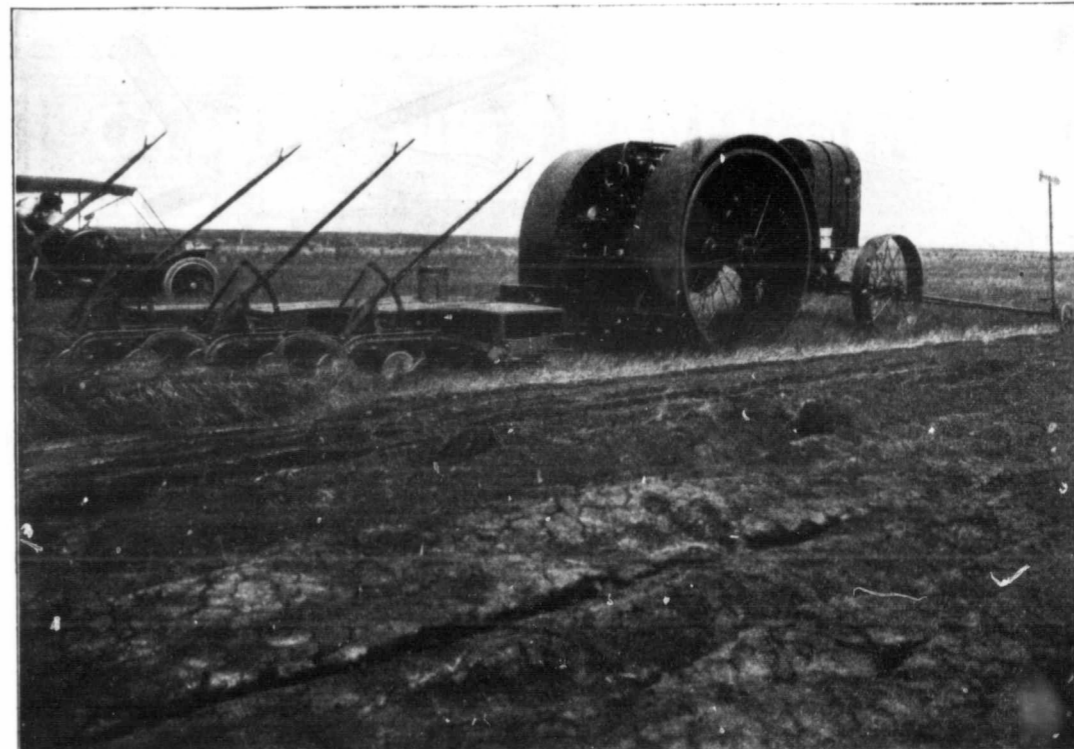
As it was pulled at the Winnipeg Motor Contest by a Gas Traction 30 Horse Power Gasoline Engine. (Gold Medal winner class C Internal Combustion Engine.) Photo taken while outfit was in motion. Note that furrow is just turning.
