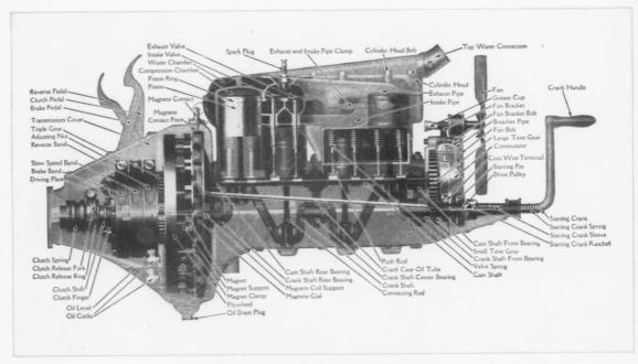
Sectional view of the Model T Motor. (Cut No. 4)
