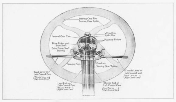
Steering Wheel Assembly showing the three reduction gears meshing with the teeth in the internal gear case and the pinner attached to the steering wheel. (Cut No. 1)
