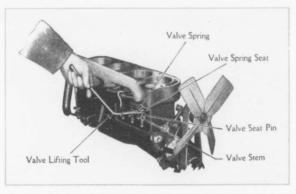
How the valve lifting tool should be used. (Cut No. 6)
