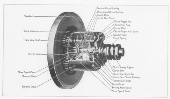
Transmission, showing all gears in mesh. (Cut No. 14)
