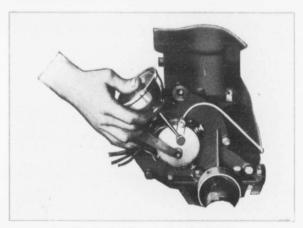
Oiling the Ford Commutator. (Cut No. 23)
