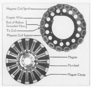
The Ford Magneto. The flywheel with magnets revolves with the engine, while magneto coils remain stationary. (Cut No. 13)
