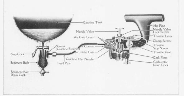
This cut illustrates the principle of Ford Carburetion. (Cut No. 9)
