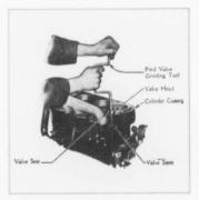
Method of grinding valve. (Cut No. 7)
