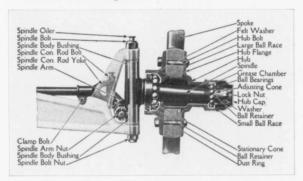
The Ford Spindle and Front Hub Assembly. (Cut No. 21)
