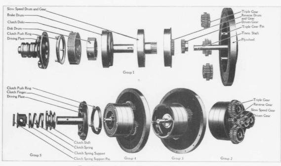
Transmission parts in their relative assembling positions. (Cut No. 17)
