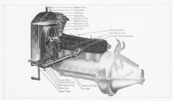
The Thermo-Syphon Cooling System of the Ford has no pump or complicated mechanism. Arrows show course of water through water passages. (Cut No. 8)
