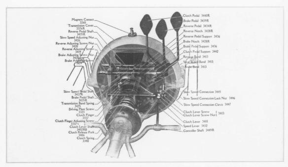
Clutch, Reverse and Brake Pedals and their Adjustments. Right Control Cars. (Cut No. 16)
