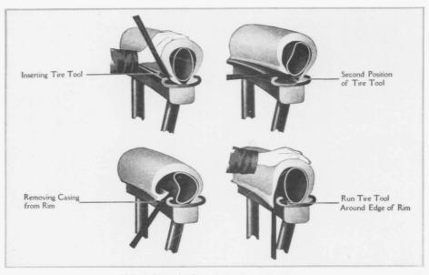
Method of removing Ford clincher tires. (Cut No. 24)
