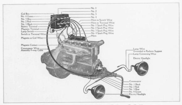
Wiring of the Ford Ignition System, also Electric Horn and Headlamps. (Cut No. 11)
