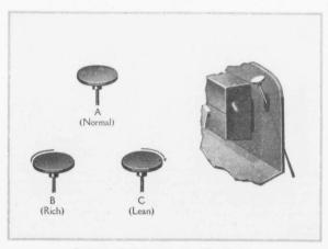
Carburetor Dash Adjustment. (Cut No. 10)
