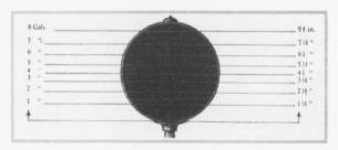
Gasoline measure for 8-gallon tank. (Cut No. 25)
