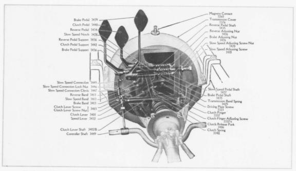
The above drawing shows the operation and adjustments of Clutch, Reverse and Brake Pedals on Left Control Cars. (Cut No. 15)
