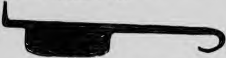
A handy grafting iron made from a blacksmith's old file.
