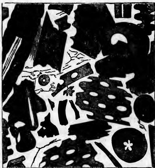
Fig. 9.—Fragment of Lower Silurian Limestone, sliced and magnified ten diameters, showing the manner in which it is made up of fragments of corals, crinoids, and shells. (From a paper on the Microscopic Structure of Canadian limestone, "Canadian Naturalist.")
