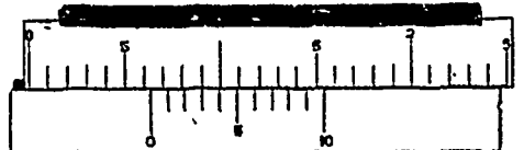
FIG. 7.—Vernier shown in Fig. 6 reading to three-tenths:
