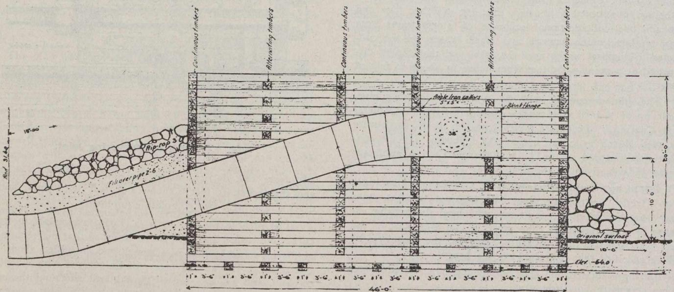
Fig. 3.—Section Through Centre of Crib and Pipe.
