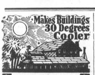
On a hot summer day the temperature in the upper part of a building covered with J-M Asbestos Ready Roofing is from 15 to 30 degrees cooler than with any other roofing. The white asbestos surface reflects the heat instead of absorbing it and transmitting it to the rooms below.
