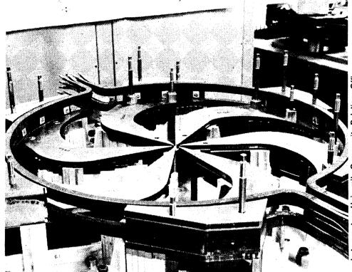
The bottom half of a 1/20 scale model of the TRIUMF magnet. View shows the contours of the
