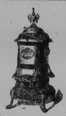
The "Enterprise Hot Blast" is a new stove on a new principle. A blast of hot air descends a tube from the top of the stove. This ignites the gases that arise from the fuel; hence one half more heat with two-thirds the usual amount of fuel.
