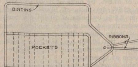
regular instrument case. Even if it is accidentally dropped, the instruments are not likely to be damaged, as they do not drop out even if the case is open. A similar accident with the other types of cases is, however, usually disastrous, as the instruments fall out and scatter all over the floor, generally with damage done to one or another of them.
