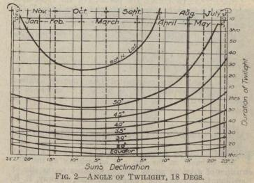
Diagram indicating the duration of twilight at various seasons of the year and at various latitudes in the northern hemisphere, assuming that the angle of twilight is 18 degs. (that is, 1 hr. 12 mins, at the equator when the declination of the sun is zero-about March 22nd and September 22nd).
