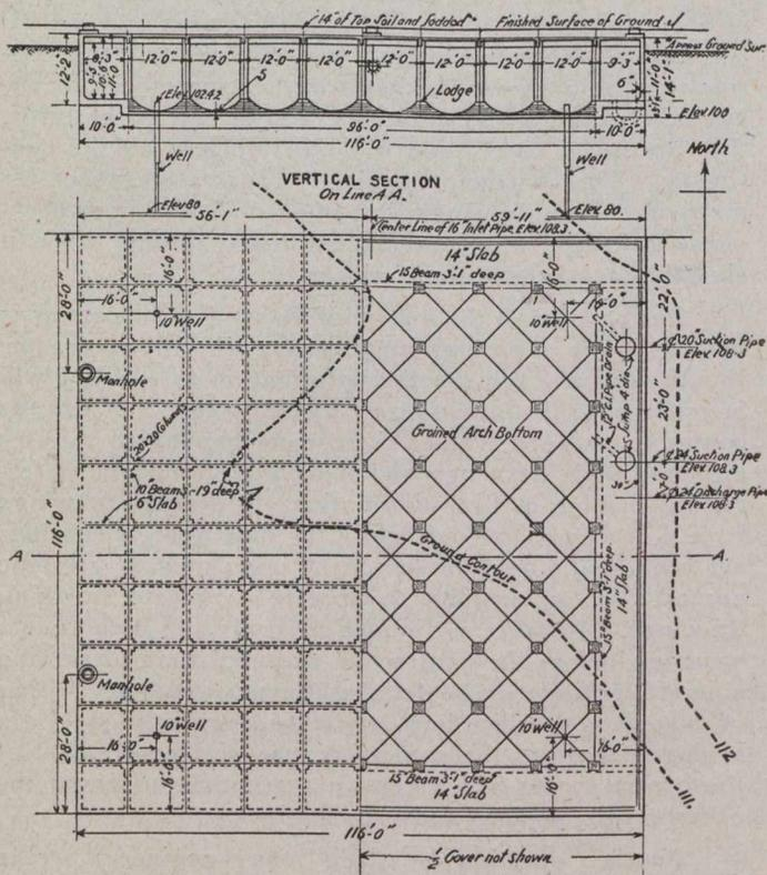
Fig. 4.—Plan and Section of 1,200,000-Gallon Covered Reservoir.
