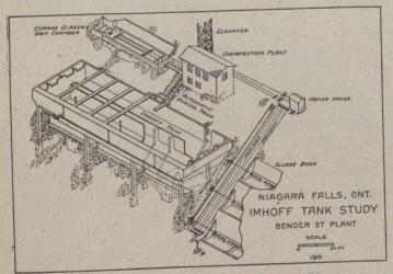
Fig. 2.-Bender Street Imhoff Tank Plant.
