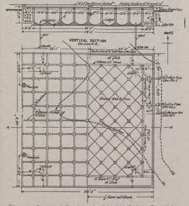
Fig. 4.—Plan and Section of 1,200,000=Gallon Covered Reservoir.
