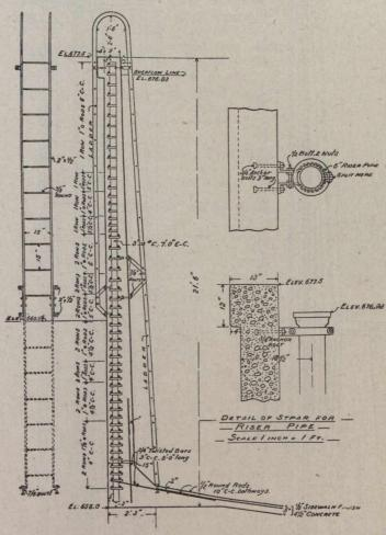
Fig. 1.-Wall of 2,000,000-Gallon Reservoir.
