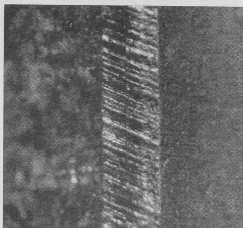
Fig. 6. A comparison of a section of the impression of a steel chisel on the iron base of a safe and the corresponding section of a test engraving made with the chisel in evidence, taken on sheet lead. The characteristics in one impression only were recorded photographically. Illustration No. 6 is one of two comparisons of items on the left bank of the evidence and test impressions. Two comparisons were also made of the items on right bank. A total of ten such comparisons was possible, but not required. Following submission of this material in evidence, the defence attorney was heard to remark that he would advise his client to leave his tools at the job in future. The culprit had pocketed the 25c chisel with the proceeds, a sum in excess of $2,000.00.
