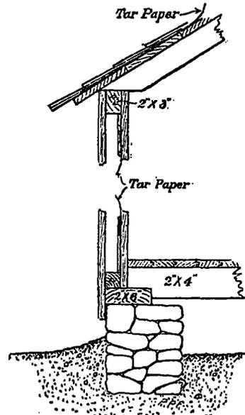
Fig. 1.—Method of building a poultry house with hollow side-walls.
