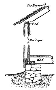
Fig. 1.—Method of building a poultry house with hollow sige-walls.
