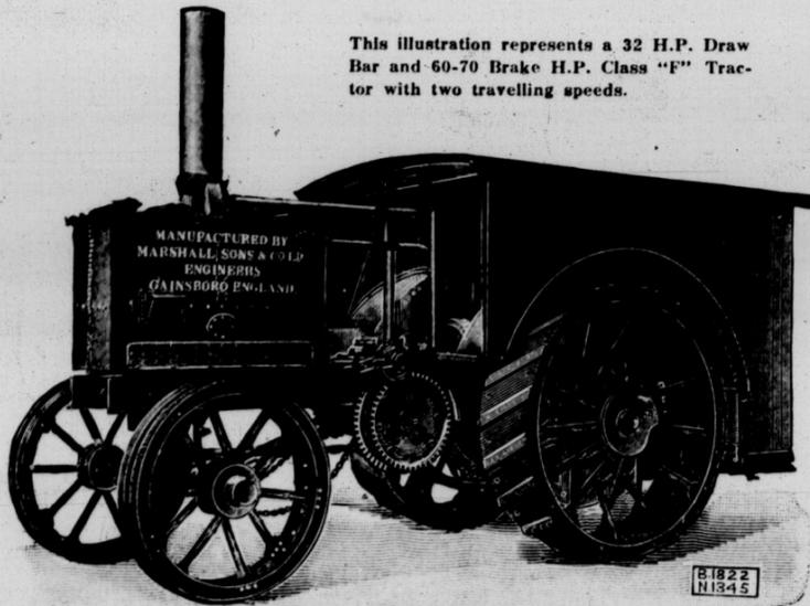
This illustration represents a 32 H.P. Draw Bar and 60-70 Brake H.P. Class "F" Tractor with two travelling speeds.
