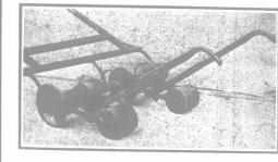
This Seeder is made both single and double, and in either form is without an equal as a compact handy implement. The seed-box is run by a friction gear, and can be stopped and started instantly without stopping the horse. It can be regulated to sow any desired quantity of turnip, mangold or carrot seed.
