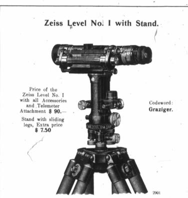
Small Level fitted with novel devices for viewing the bubble without parallax and for rapidly verifying the adjustment from a single station point (by Wild's method).
