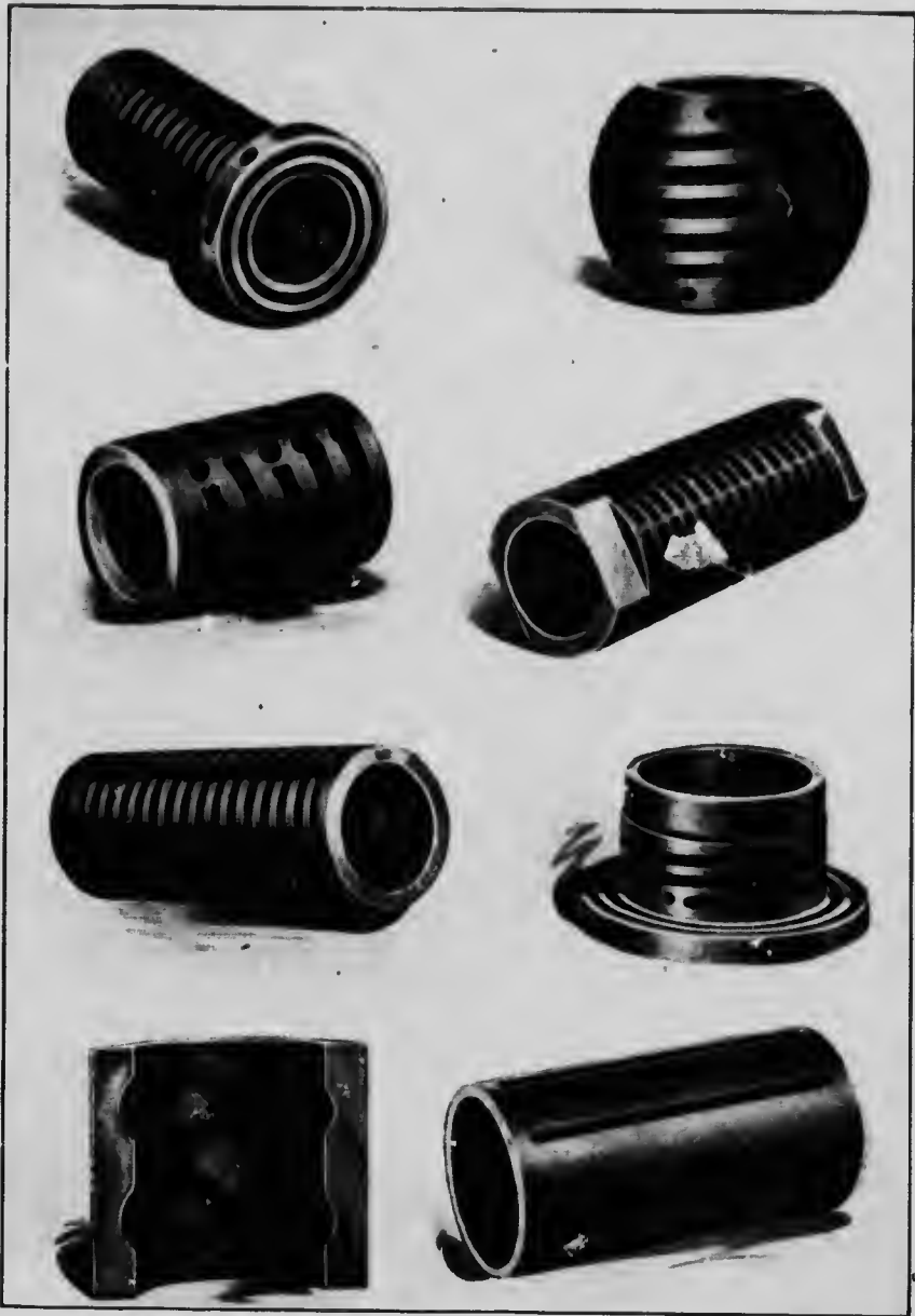
Types of Bound Brook oilless bushings. (Bound Brook Oilless Bearings Company, Bound Brook, N.J.) The bushings are cast with grooves, which are afterwards packed under hydraulic pressure with a graphite lubricating compound.
