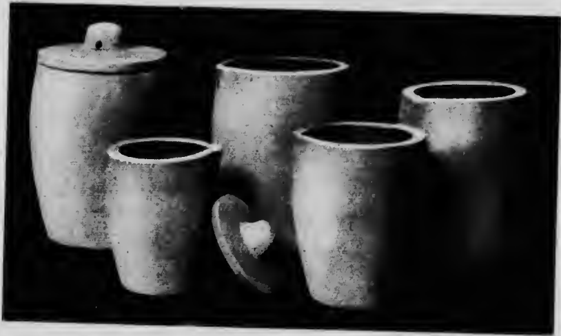
Types of crucibles used in melting non-ferrous metals. (Joseph Dixon Crucible Company, Jersey City, N.J.)
