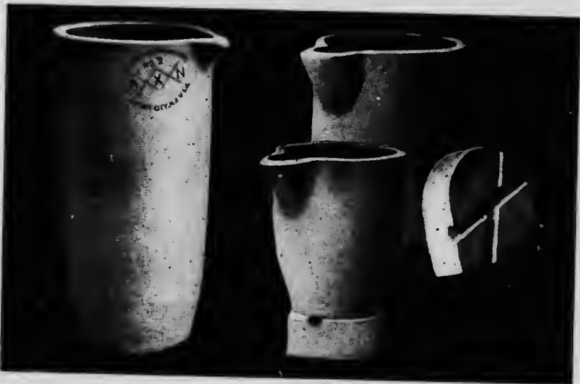
Types of crucibles used in tilting furnaces. (Joseph Dixon Crucible Company, Jersey City, N.J.)
