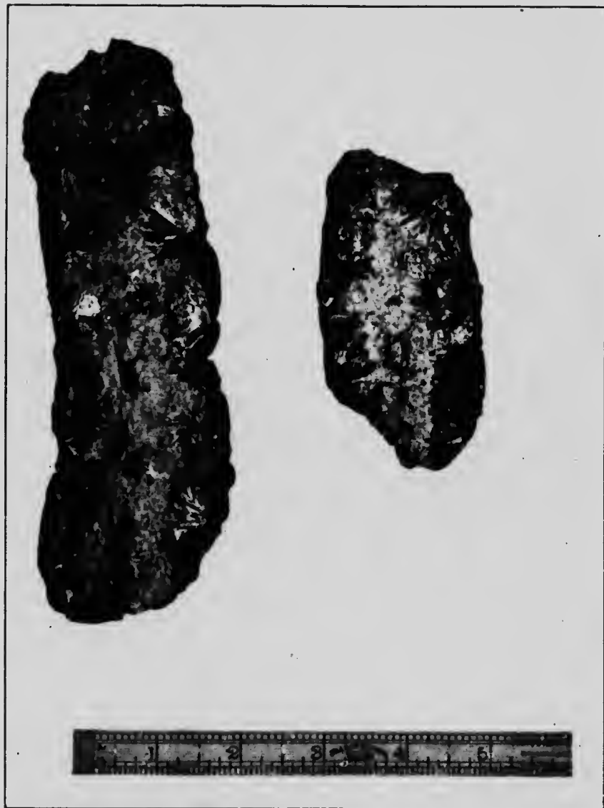
Radiated, lamellar crystals of graphite penetrating a narrow band of highly silicated limestone enclosed between two pegmatite stringers. The original limestone has been almost completely altered to a mixture of granular quartz and feldspar, with subsidiary sphene and pyroxene. From range III, township of Low, Que.
