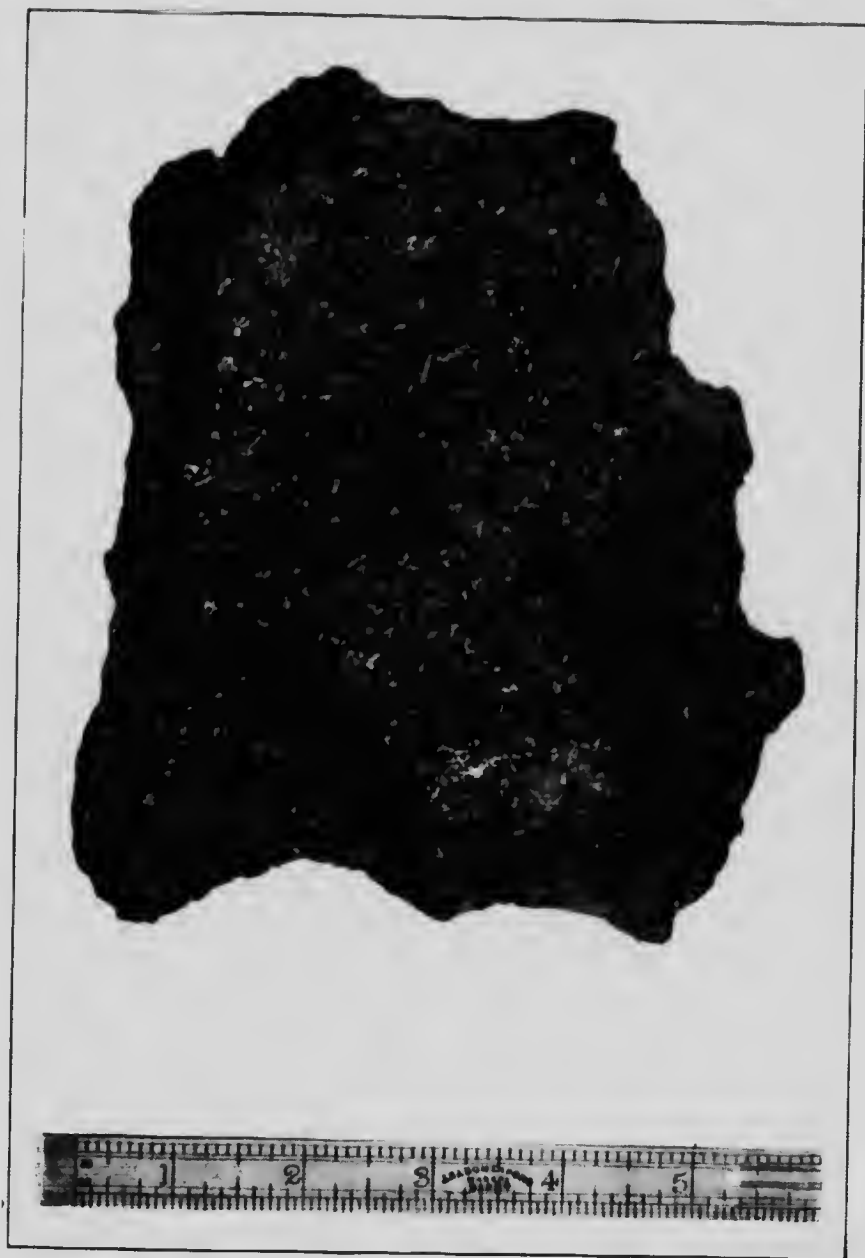
Typical high grade, Canadian flake graphite ore, 15-20 per cent carbon, from the Buckingham district, Que.
