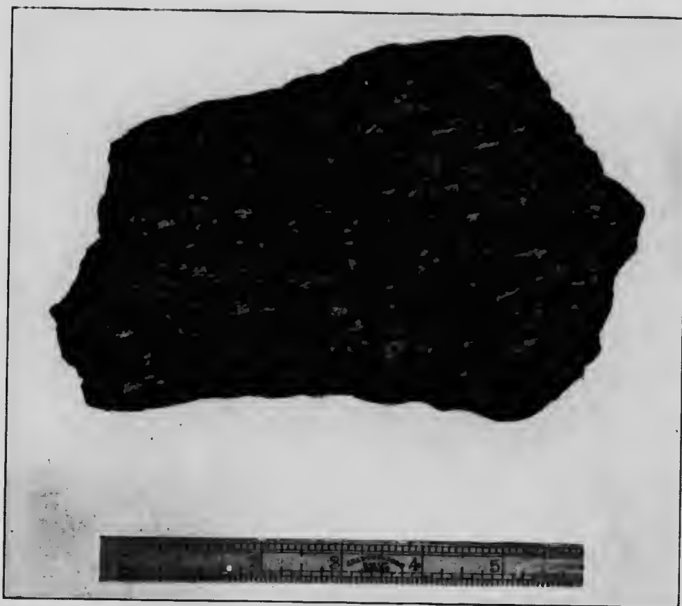
"Needle-flake" graphite ore, from concession VI, lot 21, township of North Elmsley, Ont.
