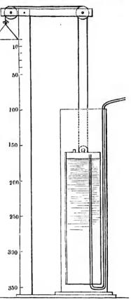
to two hundred and Spirometer used on board H. M. S. "Sophia," made from a description given in the "Lancet," vol. i. 1850.
