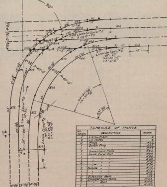
Fig. 3.—Special Work Standards for Left Hand Double Track Branch-off.
