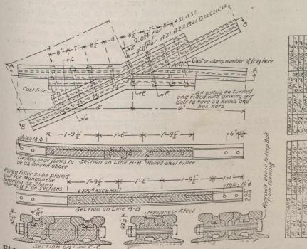
Fig. 6.—Standard Built-up Frog With Manganese Filler.
