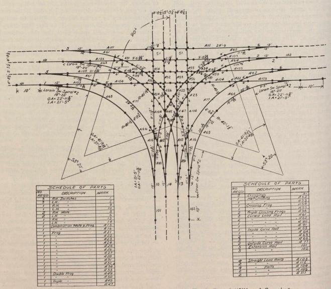
Fig. 1.-Special Work Standards for Double Track Closed "Y" and Crossing.
