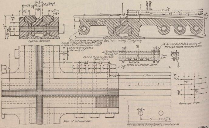
Fig. 5.-Details of Standard Double Track Crossing
