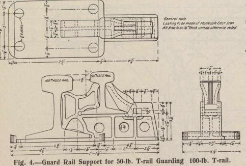
best adapted to this section was the 50-lb. T-rail. A section of this in its relation to the main rail is shown in Fig. 4, which also illustrates the standard chair
