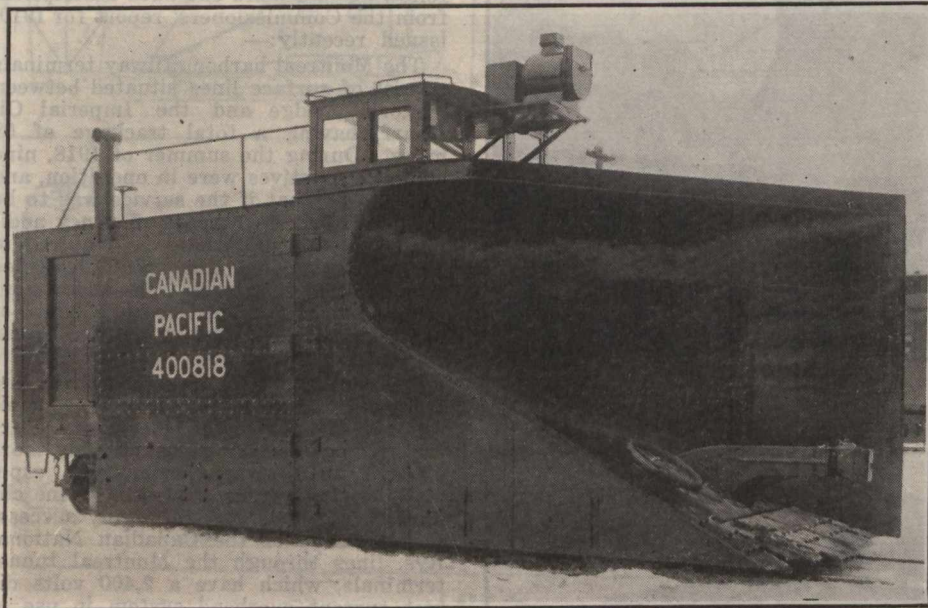
Fig. 14. Double track, steel snow plough, Canadian Pacific Railway. See page 471.
