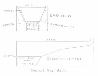
bricks for sides of the fireplace, as I think they would give more permanency to the arch. After building, we banked up the arch, and kept a fire in the cooker to keep out the frost, and watered the arch with warm water until it was well set. So we had it ready for the sap when it came. It has stood one season all right, and I don't see why it won't stand many of them.
