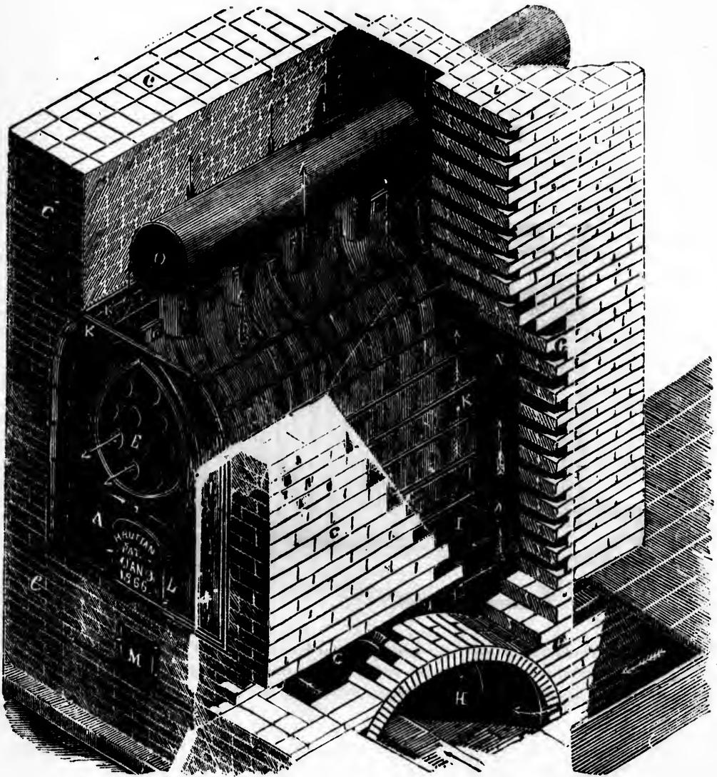
You will at once perceive that this is set in brick, and must, therefore, be set in a basement or cellar. It will warm an ordinary sized church, provided it is not too high in the ceiling, or a gaol, or asylum, or other public building. It requires for its supply eight feet, or 1152 inches of air.
