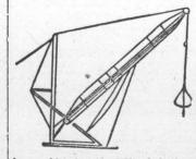
by a cable, the side drift of the boom being checked by a laterally adjusted guiding member over which the sup-porting cable is guided, is a main feature. A drum winds up and unwinds the rope or cable, which lifts the boom, one end of rope being fastened to the drum and the other to a sta-tionary support. The drum may be placed into or out of locking engagement with the guide pulley over which the hoisting is done.
