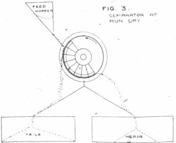
The apparatus was designed to be run either dry or wet and the drum can be rotated in either direction and at a great variety of speeds.
