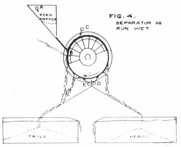
It was found that the co-efficient of friction of magnetite on brass is so low that the grains tended to accumulate in rows in front of each pole piece. This difficulty was overcome by placing a few strips of electric tape across the drum parallel to the axis. Covering the drum with canvas was also tried, but while this gave good results in dry concentration, it carried too much non-magnetic stuff when run wet.
