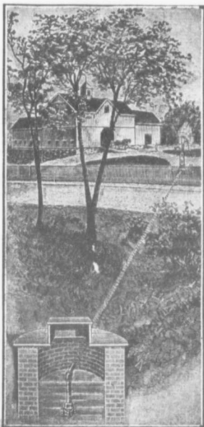
WELL CONNECTED TO PUMP IN STABLE YARD
