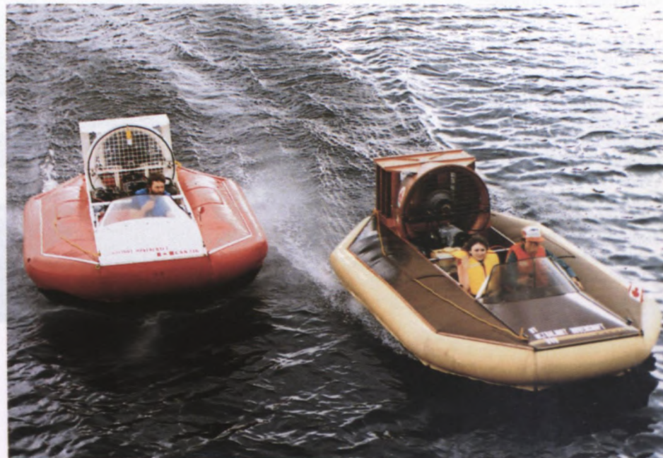
Canair 500 and 340 hovercraft with unique side-by-side seating
