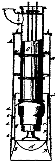
22787 Andrews' Well and Reservoir for Procuring Water from the Earth.
