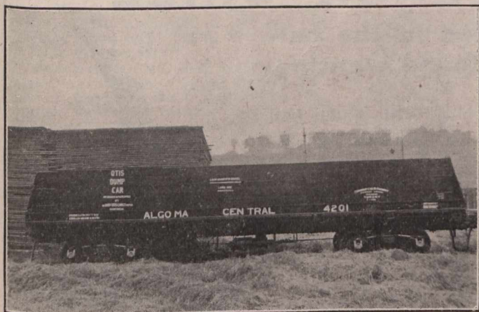
Otis Composite General Service Cars, built for the Algoma Central and Hudson Bay Railway.
