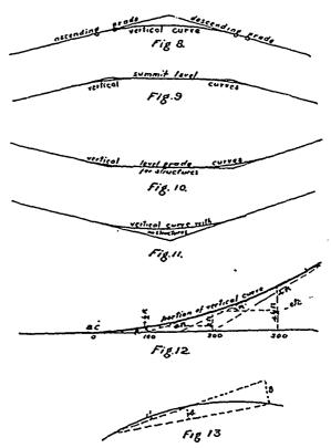
united to a level or ascending grade, an accurate calculation should be made for reasons already given. For instance, supposing that the longest train on the road will be 500 feet (engine and 14 cars), then
