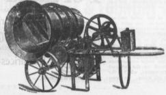
These machines are made to mix either continuously or in batches, and can be operated either by Hand, Steam or Gasoine Power.
