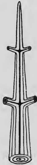
FIG. 5.—Diagram showing the connection of all branches with the pith.
