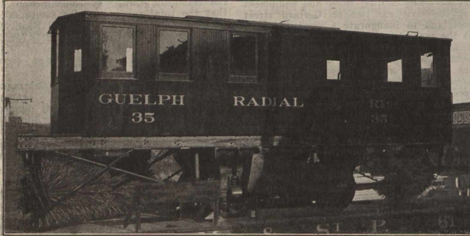
Double End, Single Truck Snow Sweeper, for Guelph Radial Railway.
