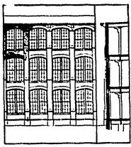
CONSTRUCTION OF FACTORY DEVISED BY EDWARD ATKINSON, THE PURPOSE BLING TO CONSTRUCT THE ALLEYWAYS SO THAT THEY SHALL BECOME HORIZONTAL TRUSSES, TO PREATEST THE VIBRATION OF THE STRUCTURE.
