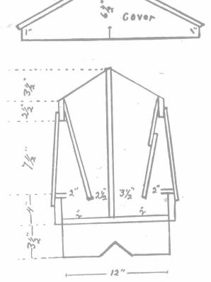
Top and End View of a Feed Hopper.
