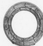
End View of Pipe and Coupling.
