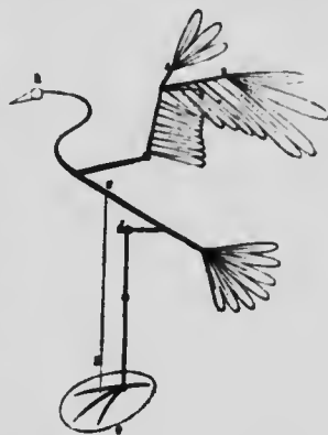
FIG. 298. — PLAN OF BIRD. s, center of gravity.
