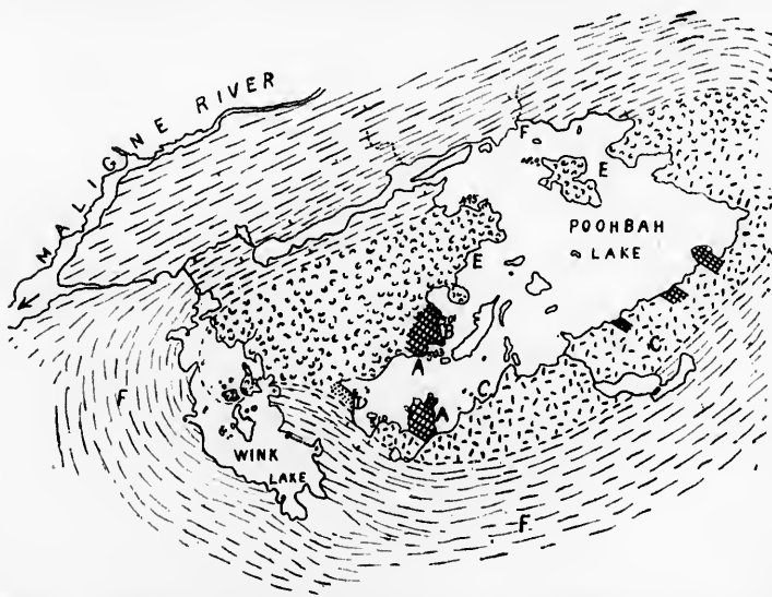
FIGURE 1.—Sketch map of Poohbah Lake; showing relation of the laccolite mass to the Couthiching schists. A, nepheline-pyroxene-malignite; B, panidiomorphic-gneissic-facies of the same; C, garnet-pyroxene-malignite; D, a minor facies of the same; E, amphibole-malignite; F, Couthiching schists. The numbers 495, 501, 503, 506, and 510 indicate where specimens were taken. Scale, two miles=one inch.
