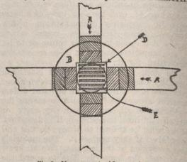
Fig. 3.—Measurements of Incenerator A. Trenches—Length 12 ft, depth 14 ins, width 12 to 14 ins.
