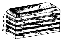
34219 Hallwood's Street Pavement.
